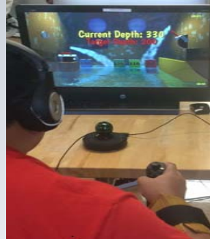
Figure 1: BrightBrainer Virtual Reality (BBVR™) system. The BBVR system features a Razer Hydra magnetic motion-sensing hub that simultaneously tracks the exact location and orientation of two controllers in three dimensional space. The BBVR™ Active Treatment program contains 11 games that offer cognitive and motor therapy as well as positive reinforcement using both visual and auditory cues. Participants in the active treatment program complete 3 sessions per week for 6 weeks.
